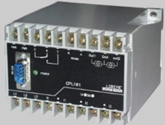
The CPL101 is a programmable transmitter designed for electrical network measurement. It covers the whole network wiring configuration met in industrial environment. It's various outputs types, allow to use it as analyser, converter, energy counter or in monitoring or protection.
